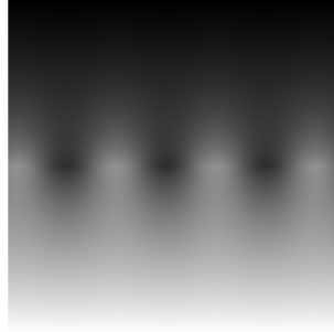
Fig. 5.5. A Rayleigh-Taylor mode on a density gradient. This grayscale representation shows a vertically exponential density profile in which there is a density perturbation due to a single mode
